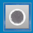
When the ink was injected through the NanoCeram® filter, the back pressure was low and filtration was easy. Yet the effluent came out water white. The filter (above) was intensely colored, proving that it retained the nano ink.
