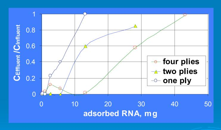
DNA and RNA are filtered much like virus. The thicker the filter, the higher is its filtration efficiency.
