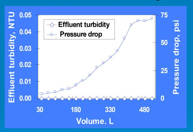
A 5" cartridge was challenged by 250 NTU of fine test dust (equivalent to a very muddy river) at 1.5 gallons/min. At end of test it had filtered out ¼ pound of dust, removing it all (>99.996%). A significant application is the sampling of municipal, well water and seawater for virus contamination
