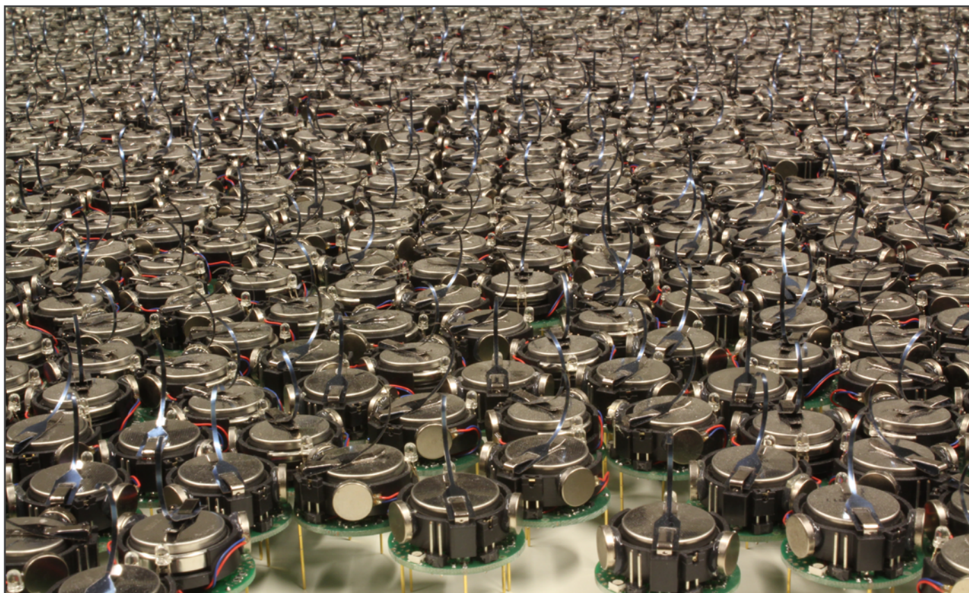
Kilobot is a thousand robot swarm developed at Harvard University, Wikimedia Commons.
