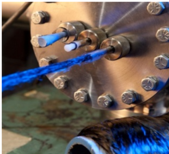
Carbon Fiber from Microwave Assisted Plasma (MAP)
